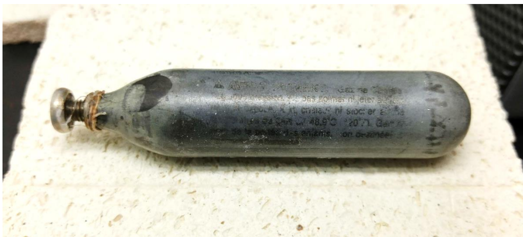
Fig 4. Threaded CO 2 cell used for the thermal decomposition of ferrocene
