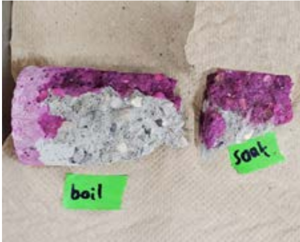
Figure 7: Results of the Phenolphthalein Penetration Test.
