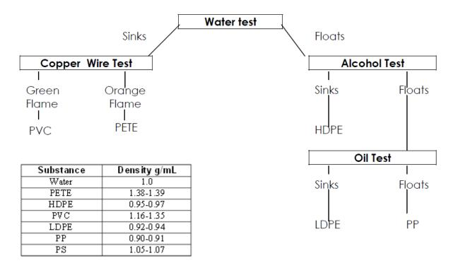
Obtain a set of samples of the seven unknown plastics (A through G). Note that each type of resin is a different shape or color. This allows for visual identification in this experiment. Actual resins may be almost any color depending on colorants added during its initial formulation.
