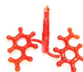
Figure 5: (Left) full part including the sprue and runners. (Right) Toyo TI-35G2 injection molding machine used to process the suspension polymer.
