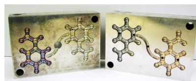
Figure 4: Core (left) and cavity (right) halves of key chain mold
